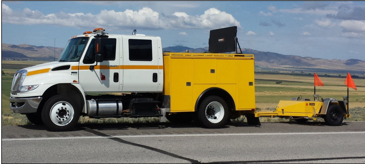
PHOTO 4: ITD'S CURRENT SKID TRUCK
