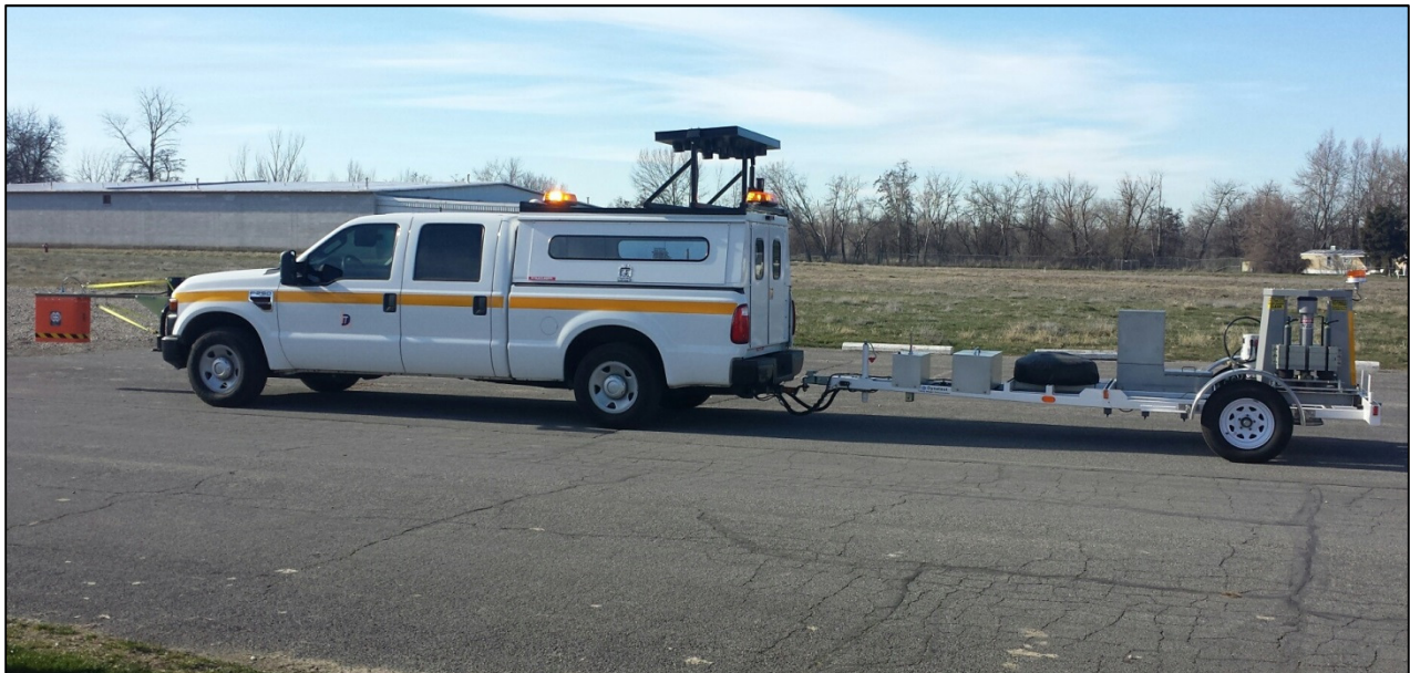
PHOTO 5: ITD'S CURRENT FWD TRUCK AND TRAILER (WITH GPR HORN ANTENNA MOUNTED TO THE FRONT BUMPER).
